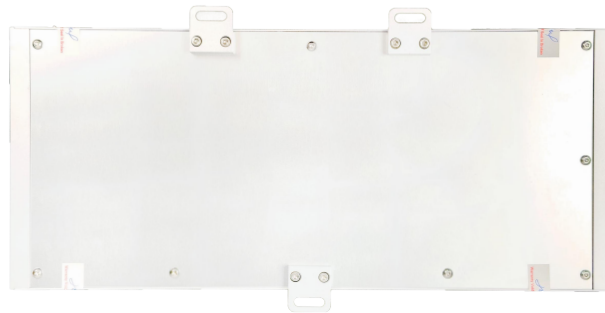
Bottom view of the laser after the fixed feet are installed ▲
